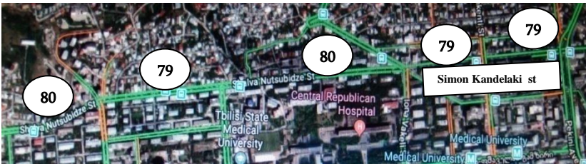
Fig. 3. The map of Shalva Nutsubidze and Simon Kandelaki streets (one-way traffic) with indicated L_{Aeq} maximum values.
